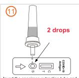
Invert the specimen extraction tube and add 2 drops of extracted specimen to the sample well (s) of the test cassette.
