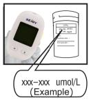
Compare the result displayed on the meter to the control solution range printed on the test strip vial. Each vial of test strips may have a different control solution range. If the results you get are not within this range, the meter and test strips may not be working properly. Repeat the control solution test.
