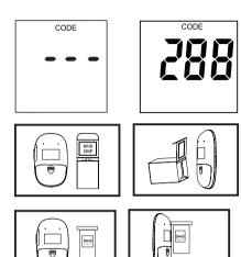
Set up the code Align the label area on the back of the uric acid instrument with the RFID on the cover of the test box. And check that the code number displayed on the screen is consistent with the code number marked on the test box.
